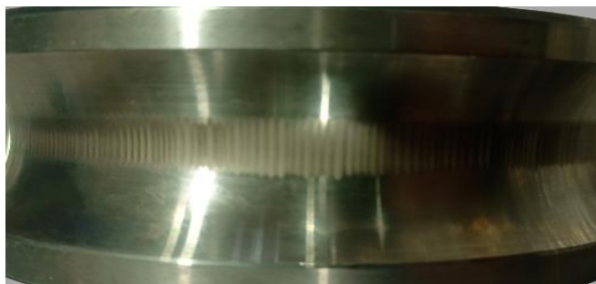
Picture 1 Bearing Fluting (courtesy of 3Phi Reliability)
