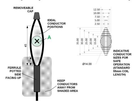
If there is a surface with a high voltage very close to the coil and the voltage is subject to high rates of change (e.g. 1kV/µs) or high frequency oscillations in the MHz range, then measurement error can arise due to capacitive coupling to the coil. For the CWTUMHF-F interference from external voltages are significantly attenuated due to the electrostatic screen that covers the Rogowski coil.
