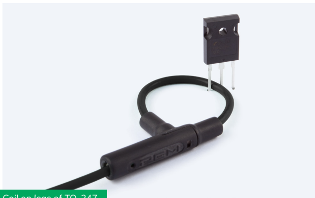
Coil on legs of TO-247
