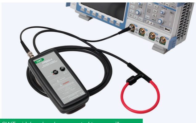
CWT wideband probe connected to an oscilloscope
