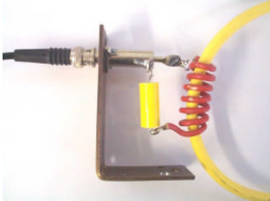
Figure 7. Photograph tuned circuit for high frequency test
