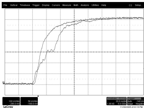
Figure 13. Test pulse \lambda=0.75 Passive transducer vs SMT current sense resistors Ch1. SMT current sense resistors 100mV/div overall sensitivity 10.0mV/A Ch2. Passive RC (54mV/div) / sensitivity 1.8mV/A Timebase: 20ns/div
