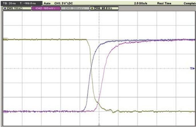
**Figure 2: A typical measurement of turn-on time in a GaN MOSFET compared with the CWTMiniHF50 probe with a co-axial shunt**
