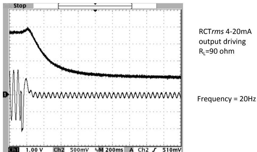
**Figure 8. Response time of 1000ms to 100% to 10% falling edge**
